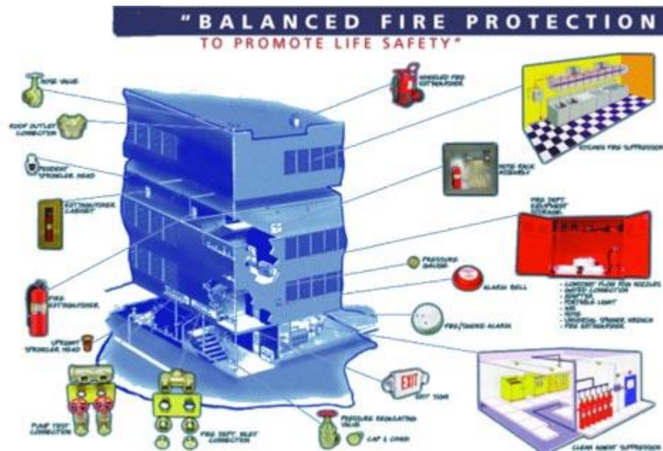
Fig7: Balanced Fire Protection
